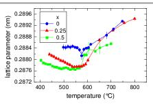
Fig. 9. Lattice parameter plotted against the annealing temperature for the  $(Fe_{1-x}Co_x)_{76}Mo_8Cu_1B_{15}$  alloy. Solid lines are only guide to the eye.
