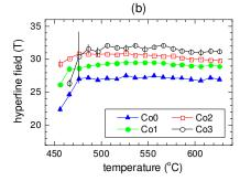
Fig. 13. Hyperfine magnetic fields of the fitted components in amorphous state (a) and of individual crystalline lattice sites with zero (Co0), one (Co1), two (Co2), and three (Co3) cobalt nearest neighbours (b) plotted against the annealing temperature as obtained from the fitting of in situ NFS data of the (Fe<sub>1-x</sub>Co<sub>x</sub>)<sub>76</sub>Mo<sub>8</sub>Cu<sub>1</sub>B<sub>15</sub> (x = 0.25) alloy. Solid lines are only guide to the eye.
