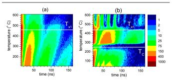
Fig. 10. Contour plot of 3-D nuclear forward scattering data of  $(\text{Fe}_{1-x}\text{Co}_x)_{76}\text{Mo}_8\text{Cu}_1\text{B}_{15}$  for x=0 (a) and x=0.25 (b). Crystallization  $T_{x1}$  and Curie  $T_C$  temperatures are indicated by the horizontal white lines.
