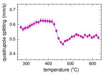
Fig. 14. Average values of quadrupole splitting of the amorphous residual matrix plotted against the annealing temperature as obtained from the fitting of in situ NFS data of the  $(Fe_{1-x}Co_x)_{76}Mo_8Cu_1B_{15}$  (x = 0.25) alloy. Solid line is only guide to
