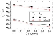
Fig. 5. Crystallization temperatures  $T_{x1}$  and  $T_{x2}$  plotted against the Co content in the (Fe<sub>1-x</sub>Co<sub>x</sub>)<sub>76</sub>Mo<sub>8</sub>Cu<sub>1</sub>B<sub>15</sub> alloys as derived from *in situ* DSR taken from both air and wheel sides of the ribbons. The lines are only guides to the eye.
