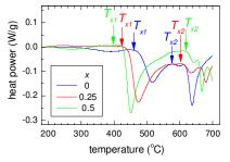
Fig. 8. Differential scanning calorimetry of the  $(Fe_{1-x}Co_x)_{76}Mo_8Cu_1B_{15}$  alloy. Temperature of the onset of crystallization is marked with arrows.
