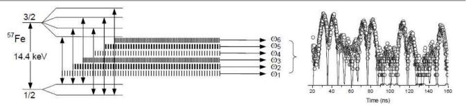
Fig. 1. Magnetically split nuclear levels of <sup>57</sup>Fe (left), photons from de-excitation transitions decays that are characterized by the frequencies (energies)  $\omega_1$  to  $\omega_6$  (middle), and the resulting interferogram (right).
