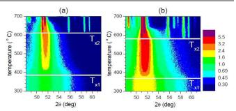
Fig. 4. Contour plots of diffractograms recorded by *in situ* DSR from the air (a) and the wheel (b) side of the  $(Fe_{1-x}Co_x)_{76}Mo_8Cu_1B_{15}$  (x = 0.5) alloy. Crystallization temperatures  $T_{x1}$  and  $T_{x2}$  are indicated by the horizontal white lines.
