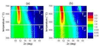
Fig. 2. Contour plots of diffractograms recorded by *in situ* DSR from the air (a) and the wheel (b) side of the  $(Fe_{1x}Co_x)_{76}Mo_8Cu_1B_{15}$  (x = 0) alloy. Crystallization temperatures  $T_{x1}$  and  $T_{x2}$  are indicated by the horizontal white lines.
