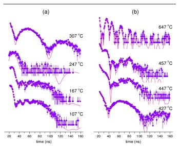
Fig. 11. Selected records obtained from NFS for the  $(Fe_{1-x}Co_x)_{76}Mo_8Cu_1B_{15}$  (x = 0.25) at the indicated temperatures in the vicinity of  $T_C$  (a) and  $T_{xz}$  (b). Experimental data (symbols) are fitted (solid lines) according to the model described in the text.
