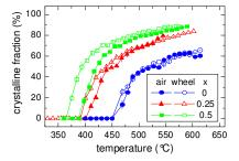
Fig. 6. Crystalline fraction plotted against the temperature of annealing as obtained from the deconvolution of *in situ* DSR data recorded from the air (full symbols) and the wheel (open symbols) sides of the  $(Fe_{1-x}Co_x)_{76}Mo_8Cu_1B_{15}$  alloy. Solid lines are only guide to the eye.
