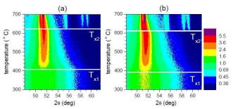
Fig. 3. Contour plots of diffractograms recorded by *in situ* DSR from the air (a) and the wheel (b) side of the  $(Fe_{1-x}Co_x)_{76}Mo_8Cu_1B_{15}$  (x = 0.25) alloy. Crystallization temperatures  $T_{x1}$  and  $T_{x2}$  are indicated by the horizontal white lines.
