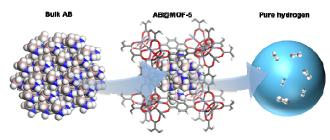
Scheme 1 The schematic structure of the confined AB-encapsulated inside the MOF-5(AB@MOF-5). The AB@MOF-5 releases pure 60 hydrogen.
