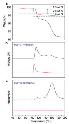
Fig. 2 Thermal decomposition properties of bulk AB (black lines) and AB@MOF-5 (red lines) samples: a. TGA spectra, b. MS for m/e=2 (hydrogen), c. MS for m/e=80 (borazine)
