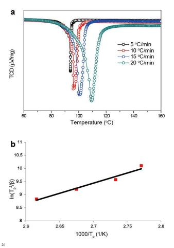
Fig. 3 a. The Temperature programed desorption (TPD) spectrum of the AB@MOF-5. b. The hydrogen desorption kinetics from Amenomiya equation.
