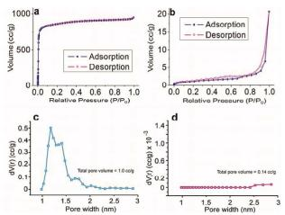
$_{15}$  Fig. 1  $N_2$  adsorption (blue) and desorption (pink) isotherms at 77 K of a. the MOF-5 and b. the AB@MOF-5. Pore size distribution of c. the MOF-5 and d. the AB@MOF-5.
