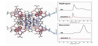
The ammonia borane-encapsulated metal-organic framework-5 enables to provide the improved characteristics, where the MOF-5 acts as a chemical guide to control the hydrogen desorption reaction pathway.
