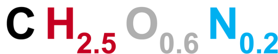
Fig. 5 Average sum formula of all products produced by the BASF Verbund. The calculation is a mass-based average, based on the annual 2024 data from the global BASF production network. It was evaluated by extracting data from the enterprise resource planning system, capturing 93% of the production.
