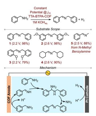
**Fig. 3** Substrate scope of TTA-BTPA-COF catalysed selective oxidation of amines. Plausible mechanism for the electrocatalytic oxidative coupling of benzylamines into *N*-benzyl-1-phenyl-methanimines by TTA-BTPA-COF.
