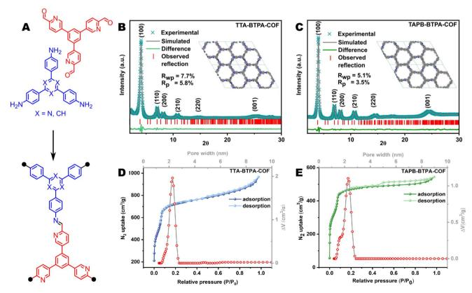
Fig. 1 (A) Synthetic scheme of TTA-BTPA-COF and TAPB-BTPA-COF. The PXRD patterns with corresponding simulated diffractogram and Pawley refinements of (B) TTA-BTPA-COF and (C) TAPB-BTPA-COF. N<sub>2</sub> sorption isotherms and pore size distribution of (D) TTA-BTPA-COF and (E) TAPB-BTPA-COF.
