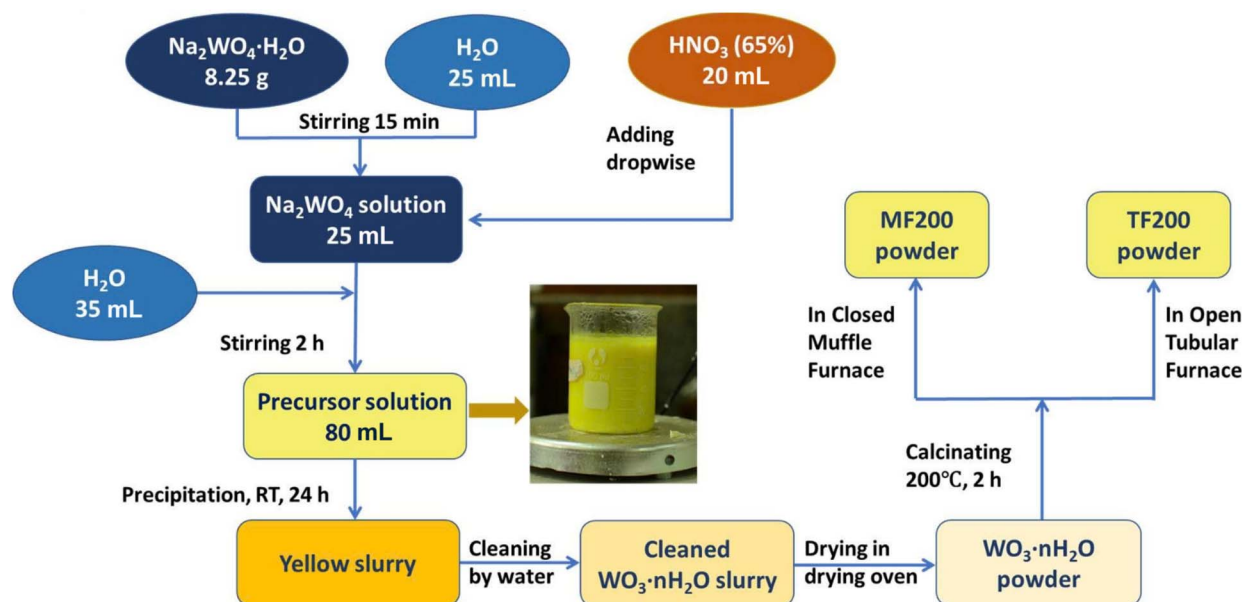
Fig. 1 Schematic of the synthesis process of cubic and monoclinic WO 3 nanostructures.
