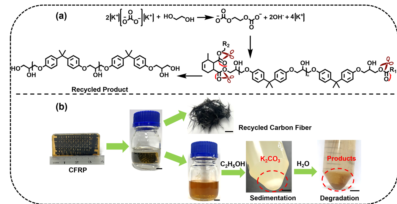
Fig. 5 (a) Schematic diagram of ester bond cleavage and (b) nondestructive recovery of carbon fibers from the composite materials. Scale bars: 1 cm.
