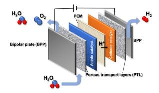
Fig. 1 Illustration of a single cell used in PEM water electrolysis.
