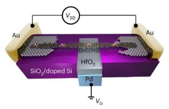
Fig. 7 Scheme of the electronic devices, where a single strand of PGNR (7.4) bridges two graphene electrodes (separated by a nanogap) connected to gold pads. A palladium gate is deposited on the SiO<sub>2</sub>/Si surface and covered with a 10-nm-thick HfO<sub>2</sub> dielectric.<sup>66</sup> Reproduced from ref. 66 with permission from [Springer], copyright [2024].
