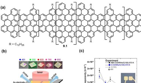
Fig. 11 (a) GNR heterostructures (9.1) synthesized for use in molecular diodes (b) Schematic I-V measurement of GNR-based device (100) (c) Average photoresponsivity of six GNR-based devices on diamond at 573 K and -5 V under vacuum conditions. 71 Reproduced from ref. 71 with permission from [ACS], copyright [2023].
