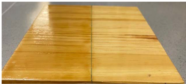
Chart 3 Application of PUD on wood. LPO-PUD (left) and PUD reference (right).
