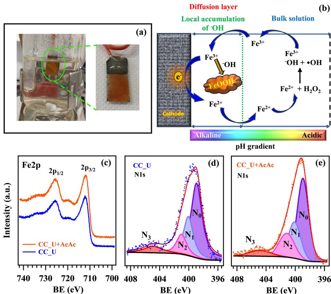
Fig. 8 (a) Image of the CC\_U + AcAc sample after the test for 24 h as a working electrode in EF processes for FNT degradation. (b) Sketch of the route yielding insoluble Fe(III) deposits onto the electrode's surface. XPS signals after EF tests for Fe2p (c) and N1s (d and e).
