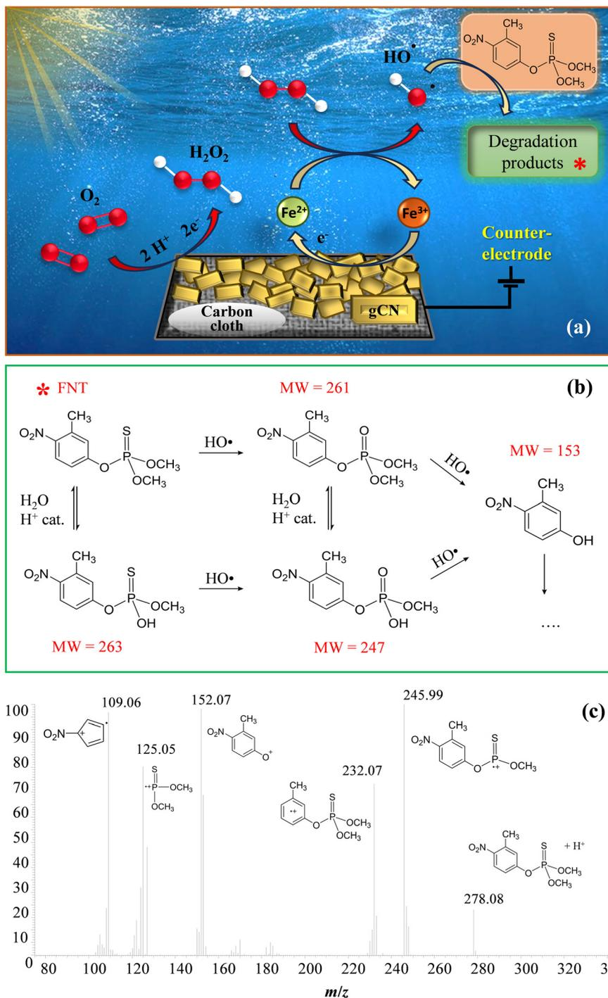
**Fig. 5** (a) Sketch of the reactions involved in the electro-Fenton process for FNT degradation. (b) Possible FNT degradation pathways and labelling of the species found in solution under the adopted conditions (MW = molecular weight). (c) Representative ESI- $MS^2$  fragmentation spectrum for FNT.
