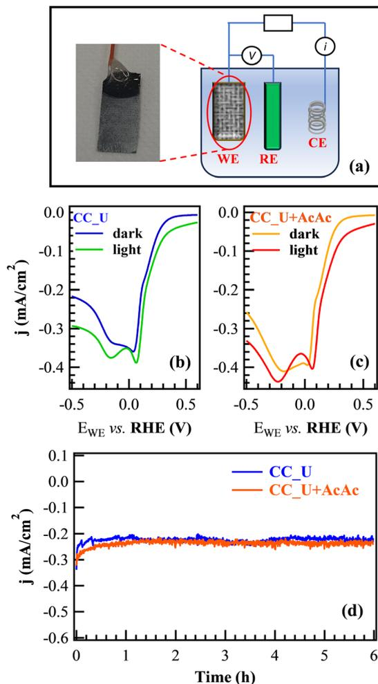
**Fig. 4** (a) Diagram of the cell used for electrochemical tests (WE = working electrode; RE = reference electrode; CE = counter-electrode). (b and c) LSV in the dark and under illumination for CC\_U and CC\_U + AcAc. (d) CA curves recorded at a bias of +0.06 V vs. the reversible hydrogen electrode (RHE).
