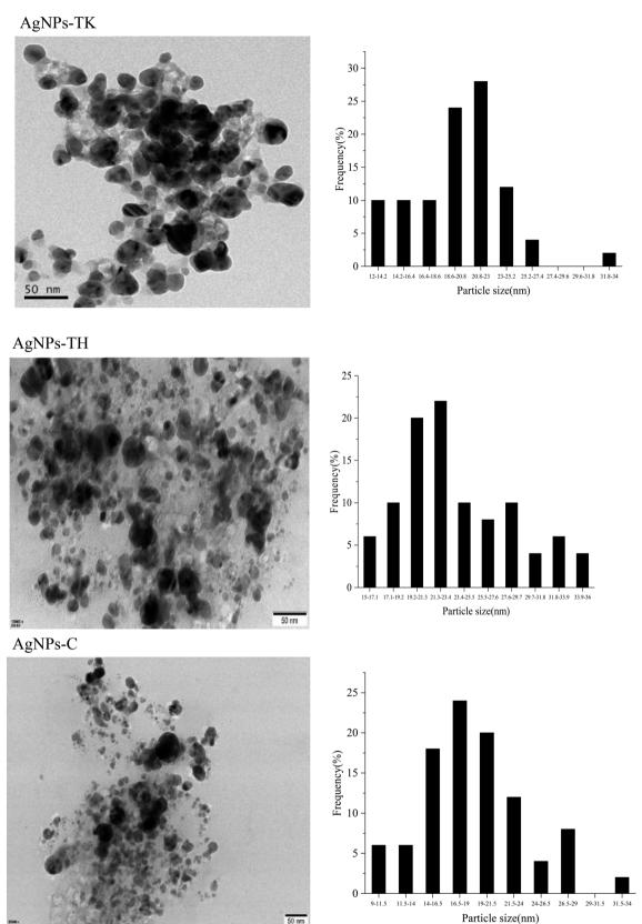
Fig. 8 Transmission electron micrographs of AgNPs (left) and particle diameter distribution of AgNPs (right).
