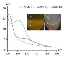
Fig. 4 UV-vis spectra of three AgNPs. The inset shows the color change of the reaction solution.
