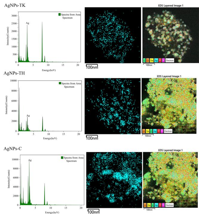
Fig. 6 EDS spectra of three kinds of AgNPs (left), and distribution of silver (middle) and other elements in elemental mapping (right).
