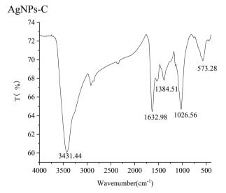
Fig. 7 Fourier-transform infrared absorption spectra of three kinds of AgNPs.
