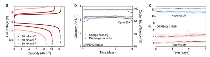
Fig. 3 Operation of a CEM pH-decoupling ARFB. (a) Galvanostatic charge-discharge voltage-capacity profile for the DPPEAQ-NaBr cell. Capacity is reported in Ampere-hours per liter of negolyte. (b) Charge capacity, discharge capacity and Coulombic efficiency of the cell during CCCV cycling under nitrogen. (c) Negolyte and posolyte pH during CCCV cycling shown in (b).
