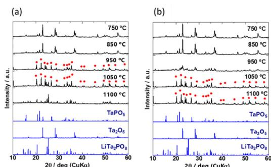
Fig. 2 XRD patterns of (a) sample A and (b) sample D after heating for 30 min at 750, 850, 950, 1050, and 1100 °C. Bottom: Simulated reference patterns based on ICSD for TaPO<sub>5</sub> (#202041), Ta<sub>2</sub>O<sub>5</sub> (#9112), and LiTa<sub>2</sub>PO<sub>8</sub> (#110781). The peaks indicated by red circles are attributed to LTPO-Precursor in this study.
