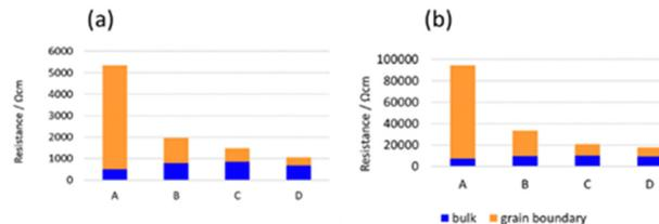
Fig. 8 Bulk and grain boundary resistances of samples after the 2nd heating measured at (a) 30 and (b)  $-10 \text{ °C}$ .
