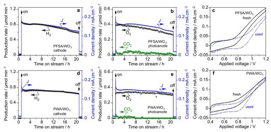
Fig. 7 Long-term stability test of (a) – (c) PFSA/WO<sub>3</sub> and (d) – (f) PWA/WO<sub>3</sub> photoanodes in the vapour-fed PEM-PEC system under visible light (453 nm, 12 mW cm<sup>-2</sup>, area 16 cm<sup>2</sup>) at 1.2 V (vs. Pt-CB): (a) and (d) Production rate of H<sub>2</sub> in the cathode side, (b) and (e) production rate of O<sub>2</sub> and CO<sub>2</sub> in the photoanode side, and (c) and (f) cyclic voltammograms before and after the stability test.
