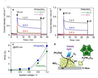
Fig. 5 Effect of applied voltage (V vs. Pt-CB cathode) on the photocurrent response of (a) PFSA/WO<sub>3</sub> and (b) PWA/WO<sub>3</sub> in the vapour-fed PEM-PEC system under visible light (453 nm, 22 mW cm<sup>-2</sup>). (c) Steady-state IPCE at 453 nm after 20 min of photoirradiation. (d) Schematic illustration of PEC triple-phase boundary over the PWA/WO<sub>3</sub> photoanode. The loading of PWA and PFSA were 5 and 12 wt% relative to WO3.
