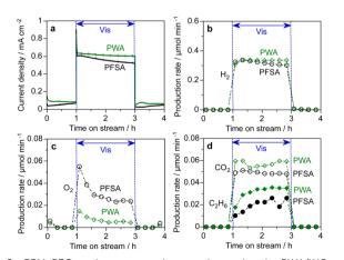
Fig. 8 PEM-PEC methane conversion reactions using the PWA/WO<sub>3</sub> and PFSA/WO<sub>3</sub> photoanodes at 1.2 V (vs. Pt-CB) under visible light irradiation (453 nm, 22 mW cm $^{-2}$ , and area 2 cm $^{2}$ ): (a) photocurrent response, (b) H<sub>2</sub> production rate at the cathode, (c) O2 production rate at the photoanode and (d) production rate of CO<sub>2</sub> and C<sub>2</sub>H<sub>6</sub> at the photoanode.
