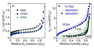
Fig. 6 (a) Nitrogen adsorption isotherms at -196 °C and (b) water vapour adsorption-desorption isotherms at 25 °C for bare WO<sub>3</sub>, PWA/WO<sub>3</sub>, and PFSA/WO<sub>3</sub> layers on Ti felt. The loading of PWA and PFSA were 5 and 12 wt% relative to WO3.
