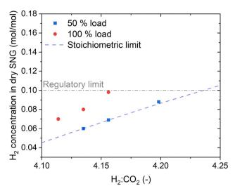
Fig. 4 The effect of stoichiometric ratio on the H<sub>2</sub> concentration in the SNG (experimental conditions: 8 bar, cooling setpoint = 230 °C).
