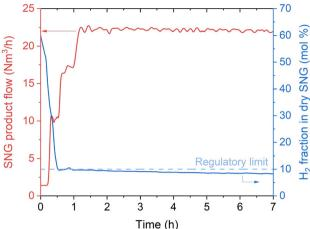
Fig. 2 Productivity and H2 fraction in SNG at the reactor outlet at the start-up of the biogas methanation plant (experimental conditions: 8 bar,  $H_2$ :  $CO_2$  = 4.15, cooling setpoint = 230 °C). The  $CO_2$  conversion is 100% in the entire time interval considered and no other products than methane were observed
