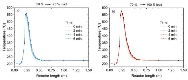
Fig. 8 Temperature profiles during the load variation: (a) from 50 to 70% load; (b) from 70 to 100% load (experimental conditions: 8 bar, H<sub>2</sub>: CO<sub>2</sub> = 4.15, cooling setpoint = 230 °C).
