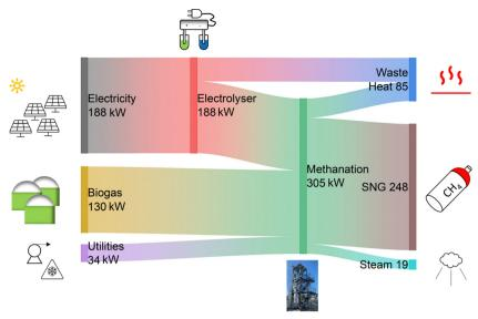
Fig. 6 Energy balance of the biogas methanation plant.
