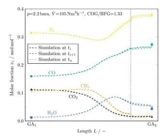
**Fig. 3** Comparison and evolution between measured data from gas analysis located at the inlet and outlet (symbols) and kinetic simulation with DETCHEM<sup>CHANNEL</sup> (dashed lines) in one syngas production phase. The vertical dotted line separates the checker chamber on the left side from the syngas main on the right side.
