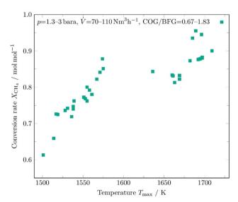
Fig. 5 Conversion rate of CH<sub>4</sub> of several syngas production phases as a function of the maximum average temperature in the reforming channel.
