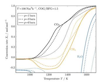
**Fig. 4** Simulated conversion rates as function of temperature at three different pressure levels predicted by DETCHEM<sup>CHANNEL</sup>.
