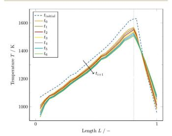
Fig. 2 Measured temperature profiles in a production phase of about 25 minutes. The time discretization  $(t_i - t_{i+1})$  used is set to 250 s.
