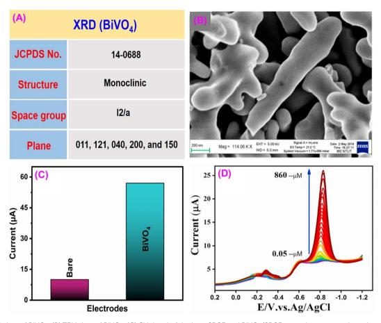
Fig. 5 (A) XRD data of BiVO<sub>4</sub>. (B) TEM data of BiVO<sub>4</sub>. (C) CV signal of the bare SPCE and BiVO<sub>4</sub>/SPCE towards paraoxon detection. (D) DPV signal of BiVO<sub>4</sub>/SPCE for detection of various concentrations of paraoxon<sup>112</sup> (modified). ((B and D) License number: 5542341491022).
