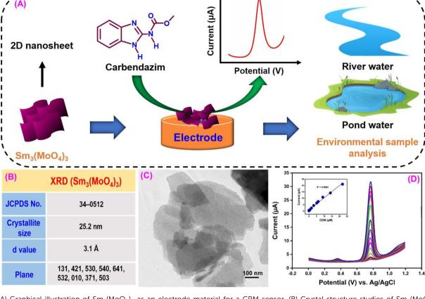
Fig. 3 (A) Graphical illustration of  $Sm_3(MoO_4)_3$  as an electrode material for a CRM sensor. (B) Crystal structure studies of  $Sm_3(MoO_4)_3$ . (C) Morphological studies of  $Sm_3(MoO_4)_3$ . (D) DPV curves of  $Sm_3(MoO_4)_3$  for CRM detection<sup>79</sup> (modified). ((C and D) License number: 5547980179571).
