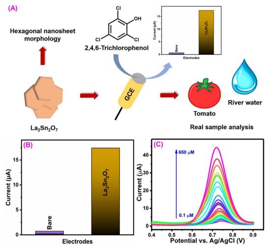
Fig. 8 (A) Schematic diagram for the synthesis of the  $La_2Sn_2O_7$  nanosheet and its electrochemical detection studies. (B) CV current response of the bare GCE and  $La_2Sn_2O_7/GCE$  towards TCL detection. (C) DPV response of  $La_2Sn_2O_7/GCE$  for detection of various concentrations of TCL<sup>124</sup> (modified). ((C) License number: 5570091012633).
