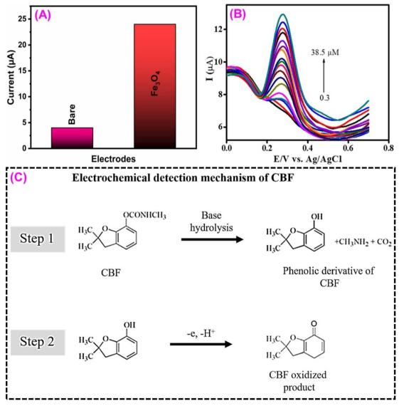
Fig. 9 (A) CV current signal of  $Fe_3O_4/MGCE$  and  $Fe_3O_4/MGCE$  towards CBF detection. (B) DPV signal of  $Fe_3O_4/MGCE$  for the CBF concentrations from 0.3-38.5 μM. (C) Possible electrochemical detection mechanism of CBF<sup>134</sup> (modified). ((B) License number: 5570091331923).
