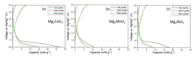
Fig. 3 Electrochemistry of Mg-rich disordered rocksalts. Charge/discharge profiles of the first three cycles of (a)  $Mg_2CoO_3$ , (b)  $Mg_2MnO_3$ , and (c)  $Mg_2NiO_3$  in Mg cells at 60 °C using 0.3 M  $Mg[B(hfip)_4]_2$  in DME as the electrolyte at a current density of 10 mA  $g^{-1}$ .
