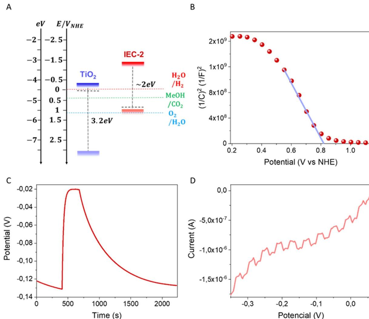
Fig. 3 (A) Band energy diagram obtained for IEC-2 (TiO<sub>2</sub> is included for comparative purposes), including the water-splitting redox couples at pH = 0 (NHE). Dotted lines represent the Fermi level positions for both materials. (B) Mott-Schottky plot of IEC-2, and (C) photovoltage and (D) linear sweep voltammetry under chopped illumination of IEC-2.
