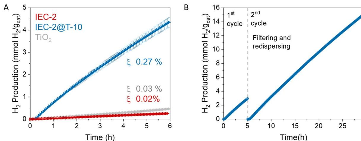
Fig. 5 (A) Cumulative H<sub>2</sub> production vs. time (h) of IEC-2 (red), IEC-2@T-10 (blue) and bare TiO<sub>2</sub> (grey) under UV illumination. Photonic efficiencies are included for reference. (B) Long duration recycling experiment using IEC-2@T-10 as the photocatalyst for H<sub>2</sub> production.
