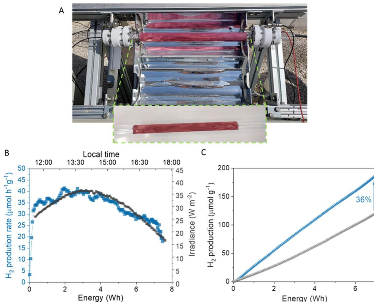
Fig. 6 (A) Semi-pilot plant solar CPC reactor and zoomed-in view of the tubular reactor coated with the IEC-2@T-10 hybrid. (B) Hydrogen evolution rate ( $\mu\text{mol h}^{-1} \text{g}^{-1}$ ) of IEC-2@T-10 vs. received solar energy. The variation of the solar irradiance (UVA) along the experiment and the elapsed time are also plotted for comparison. (C) Cumulative solar H<sub>2</sub> production of IEC-2@T-10 (blue) and bare TiO<sub>2</sub> (grey) under equivalent received energy conditions.
