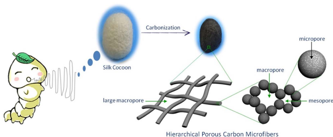
Fig. 4 Pictorial representation of preparation of hierarchical porous CMF from silk cocoon. Reproduced with permission from ref. 30 Copyright (2013), Nature Scientific Reports.
