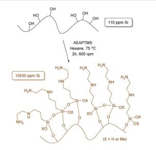
Scheme 1 Representation for the functionalization of olive stone with AEAPTMS.
