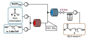
Scheme 3 Flow scheme for the acylation of 1,6-hexanediol in 2-MeTHF (3 equiv., 2.5 M) at 100 °C for 4 min with fatty acyl chloride 6 (1 equiv., crude from previous reaction) and subsequent neutralisation with aqueous NaOH (1 M, 4.4 equiv.) at 0 °C for 2 min to obtain monoester 3.
