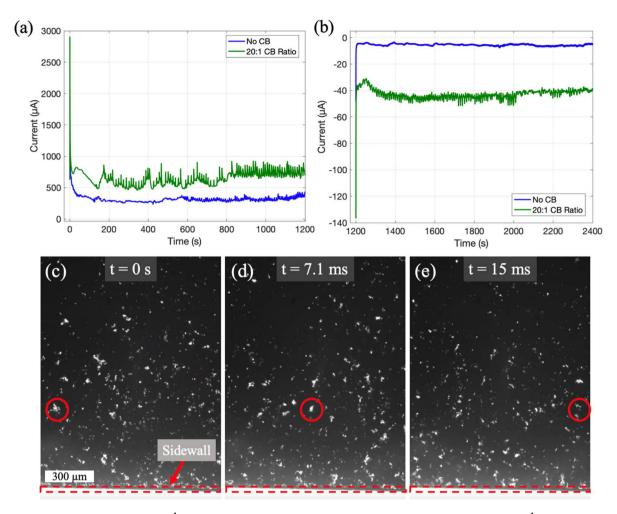
Fig. 7 (a) A comparison of the 100 μL min<sup>-1</sup> charging current with and without CB. (b) A comparison of the 100 μL min<sup>-1</sup> discharging current with and without CB. Due to the agglomeration of CB in low shear areas of the  $\mu$ -EFC, only 100  $\mu$ L min<sup>-1</sup> data could be collected. (c-e) shows still images of the carbon slurry that includes carbon black at a flowrate of 100 µL min<sup>-1</sup>.
