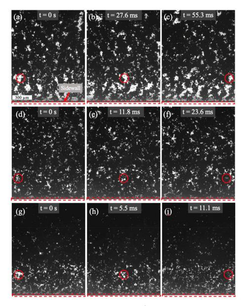
Fig. 5 Images from high-speed videos at (a-c) 35, (d-f) 50, and (g-i) 100  $\mu$ L min<sup>-1</sup> at 10 $\times$  magnification with the channel sidewall at the bottom of each image, as denoted by the dashed red lines. The red circles track a void space across the width of the view field. The scale bar in (a) also applies to (b-i) and represents 300 µm.
