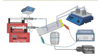
A schematic of the experimental setup including the µ-EFC, syringe pump with in-syringe mixing, an inverted microscope, a highspeed camera, a potentiostat, and outlet reservoirs.
