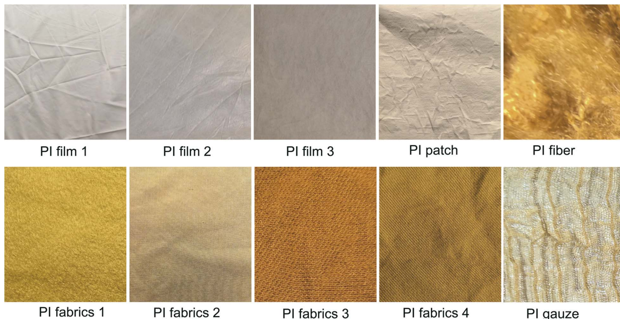
Fig. 9 Different types of PIs synthesized for the analysis of antibacterial properties. The different forms of PI tested included films, patches, fibers, fabrics, and gauze.
