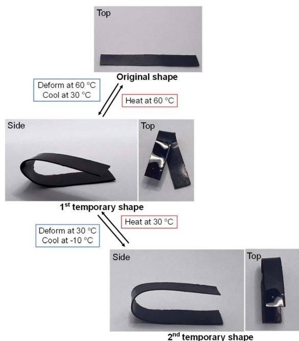
Fig. 11 Photographs of multiple-shape memory behaviours of poly(V-fa/urethane) (60/40 wt/wt).
