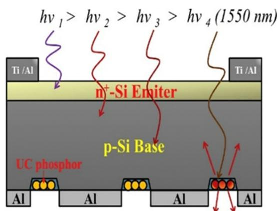
Fig. 20 A schematic diagram showing a silicon solar cell with  $\text{SiO}_2$  coating containing  $\text{YF}_3:\text{Yb}^{3+}/\text{Er}^{3+}$  phosphor particles within the backside matrix grooves for use in the upconversion of photons under excitation by a light source with a wavelength of 1550 nm. Reprinted with permission from Elsevier.<sup>77</sup>
