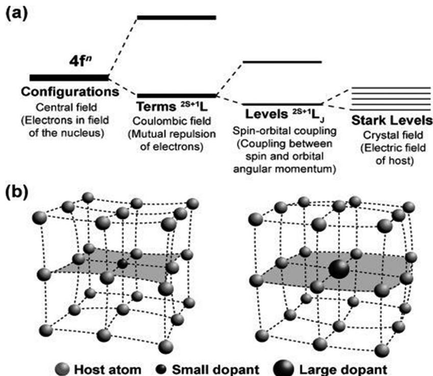
Fig. 4 (a) A simplified representation of the effect of the coulombic field, spin-orbit coupling, and crystal-field interaction on the  $[Xe]4f^n$  configuration. (b) Crystal lattice contraction (left) and expansion (right) as a result of the substitution of a host atom with dopants of varied sizes. Reprinted with permission from Wiley.<sup>53</sup>
