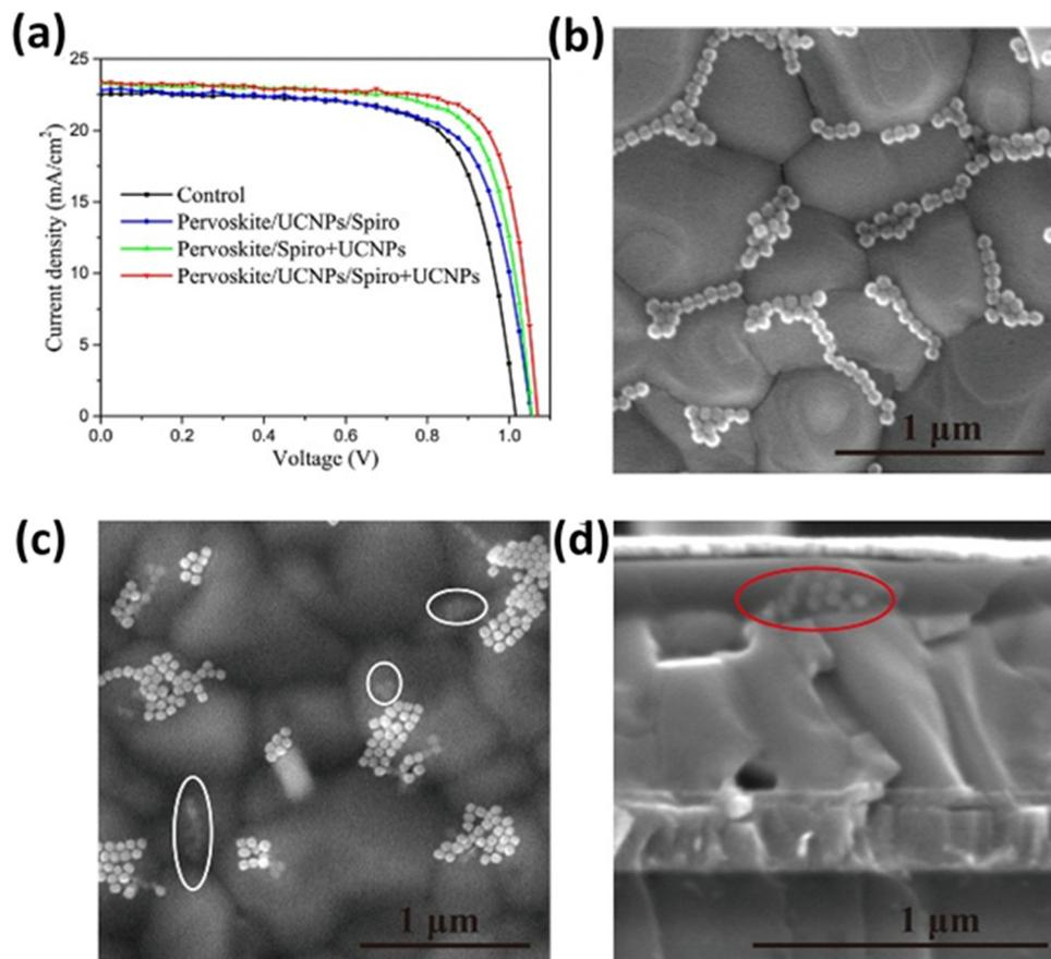
Fig. 15 (a)  $J$ - $V$  characteristics of several types of PSCs. Top-view SEM images of (b) perovskite/UCNP film and (c) perovskite/UCNP/spiro + UCNPs film. (d) Cross-sectional SEM images of the PSC with the structure of ITO/SnO<sub>2</sub>/perovskite/UCNPs/spiro + UCNPs/Au. Reprinted with permission from the American Chemical Society.<sup>93</sup>
