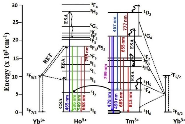
Fig. 7 Energy level diagrams of Ho<sup>3+</sup>-Yb<sup>3+</sup>-Tm<sup>3+</sup> ions and the possible UC and ET processes under 976 nm excitation. Reprinted with permission from Elsevier.<sup>60</sup>
