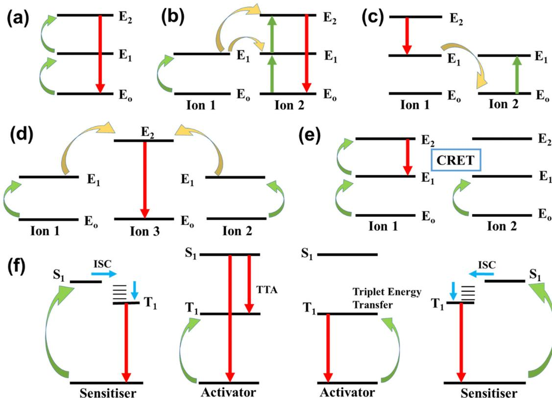
Fig. 2 Schematics of upconversion mechanisms. (a) Excited state upconversion, (b) energy transfer upconversion, (c) cross-relaxation, (d) cooperative sensitization upconversion, (e) photon avalanche, (f) triplet-triplet annihilation.
