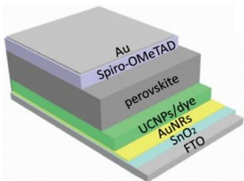
Fig. 16 The structure of PSCs and the scattering and reflecting mechanism diagram. Reprinted with permission from the American Chemical Society.<sup>74</sup>
