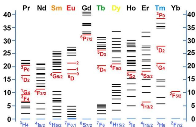
Fig. 5 Partial energy diagrams for the lanthanide aqua ions; the values of the energy levels are given as  $1000 \text{ cm}^{-1}$ . The red and blue lines indicate the main luminescence and the fundamental levels, respectively. Reprinted with permission from Elsevier.<sup>57</sup>
