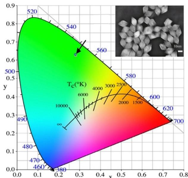
Fig. 12 The CIE chromaticity diagram of  $\text{Li}(\text{Gd},\text{Y})\text{F}_4:\text{Yb},\text{Er}$  (inset: the TEM image of  $\text{Y}^{3+}$ -doped  $\text{LiGdF}_4:\text{Yb}^{3+},\text{Er}^{3+}$  upconversion nanocrystals). Reprinted with permission from Elsevier.<sup>68</sup>
