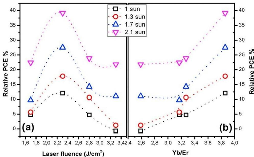
Fig. 21 The relative PCE dependence on the laser fluence (a), and (b) the Yb/Er elemental ratio measured at different solar simulator incident powers. Reprinted with permission from Elsevier.<sup>75</sup>
