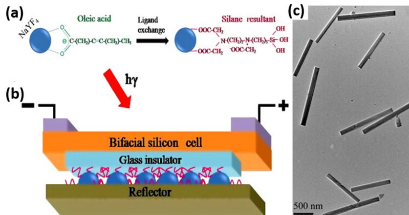
Fig. 19 (a) Ligand exchange of  $\text{NaYF}_4:\text{Er}$  nanocrystals. (b) A schematic of upconversion film application in silicon solar cells. (c) TEM image of  $\text{NaYF}_4:\text{Er}$  nanocrystals dispersed in methanol after ligand exchange. Reprinted with permission from Elsevier.<sup>76</sup>
