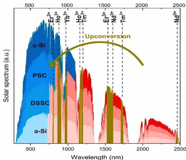
Fig. 1 Parts of the solar spectra of different solar cell types, utilized (in blue) and lost (in red), and the absorption ranges (in brown) of the upconverting  $\text{Ln}^{3+}$  ions.<sup>11</sup>
