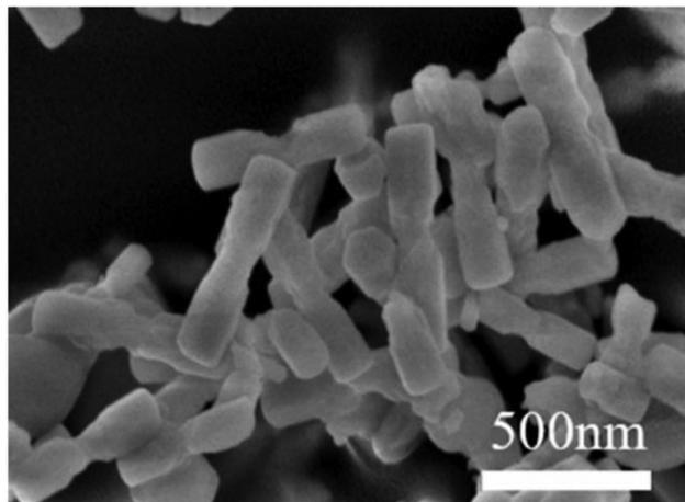
Fig. 13 SEM image of  $\text{NaGdF}_4:\text{Yb}^{3+},\text{Er}^{3+}$  nanoparticles. Reprinted with permission from Elsevier.<sup>70</sup>
