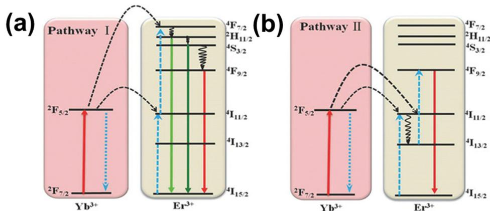
Fig. 9 The energy levels of the  $\text{Yb}^{3+}/\text{Er}^{3+}$ -codoped  $\text{NaYF}_4:\text{Yb}^{3+}/\text{Er}^{3+}@\text{YOF}:\text{Yb}^{3+}/\text{Er}^{3+}$ , showing possible energy transfer upon 980 nm excitation. Reprinted with permission from Wiley.<sup>88</sup>
