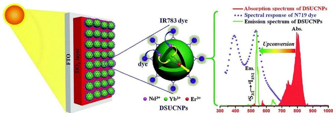
Fig. 6 Broadband near-infrared sunlight harvesting and spectral conversion into the visible range to activate the N719 dye for the improvement of a DSSC device. Reprinted with permission from Elsevier.<sup>84</sup>
