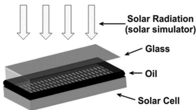
Fig. 18 A Si solar cell covered with glass and the matching oil. Reprinted with permission from Elsevier.<sup>95</sup>
