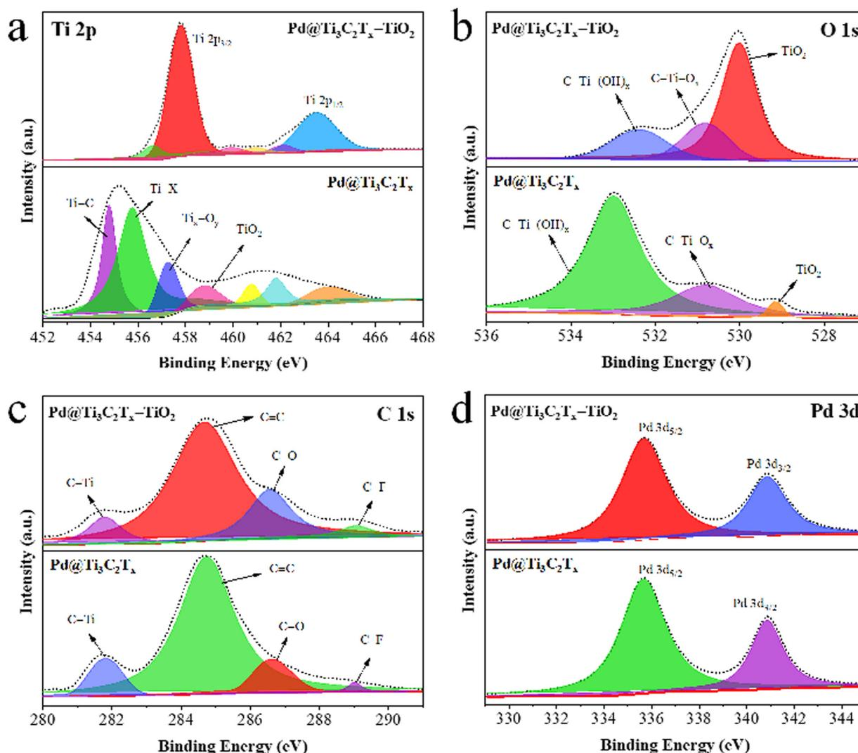
Fig. 6 XPS results of Pd@Ti<sub>3</sub>C<sub>2</sub>T<sub>x</sub> and Pd@Ti<sub>3</sub>C<sub>2</sub>T<sub>x</sub>-TiO<sub>2</sub>: (a) Ti 2p, (b) O 1s, (c) C 1s, and (d) Pd 3d.
