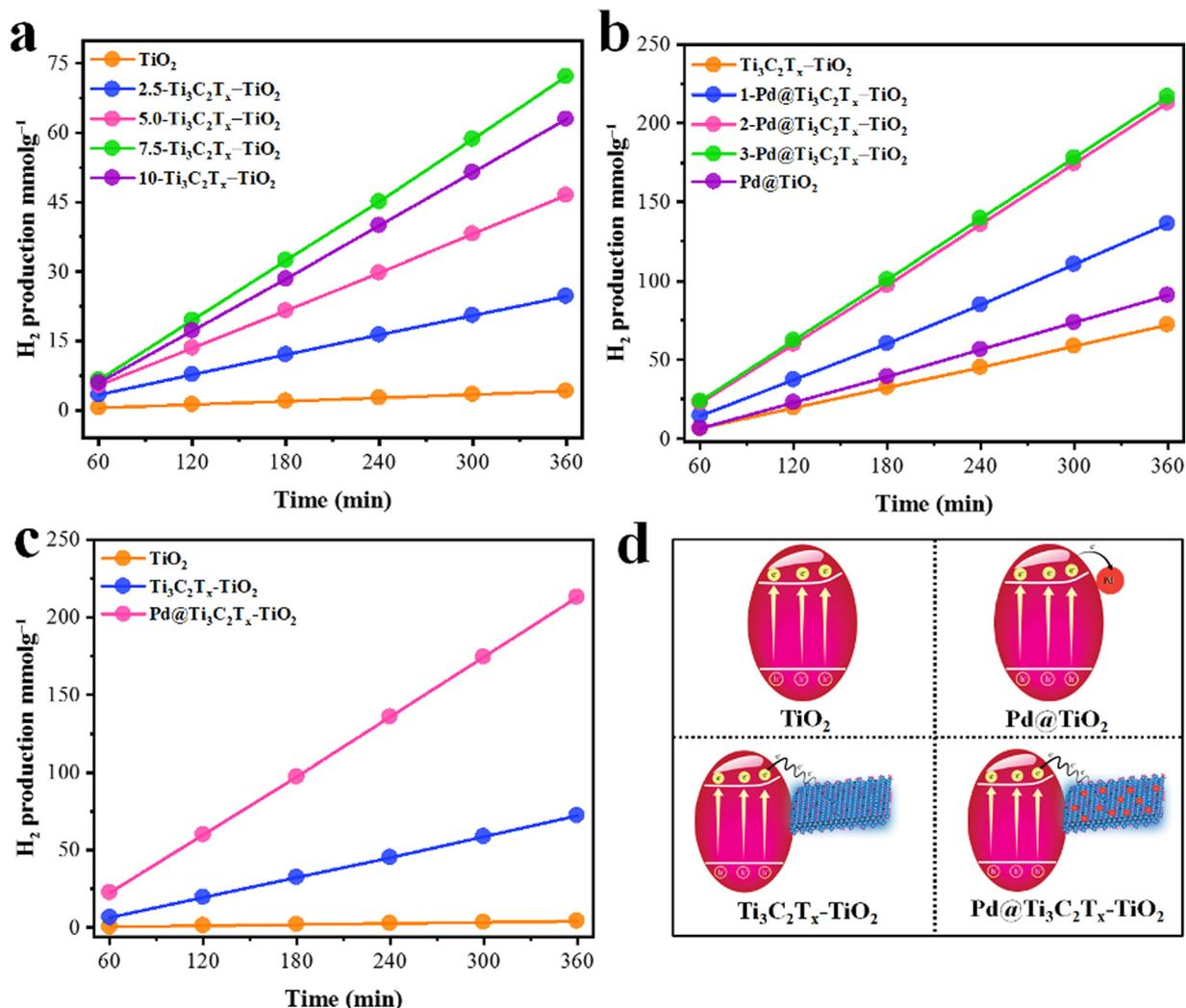
Fig. 9 (a) Optimization of  $\text{Ti}_3\text{C}_2\text{T}_x$  over  $\text{TiO}_2$ . (b) Optimization of Pd over  $\text{Ti}_3\text{C}_2\text{T}_x\text{-TiO}_2$ ; (c) comparison of optimised catalysts; (d) corresponding scheme of catalysts.
