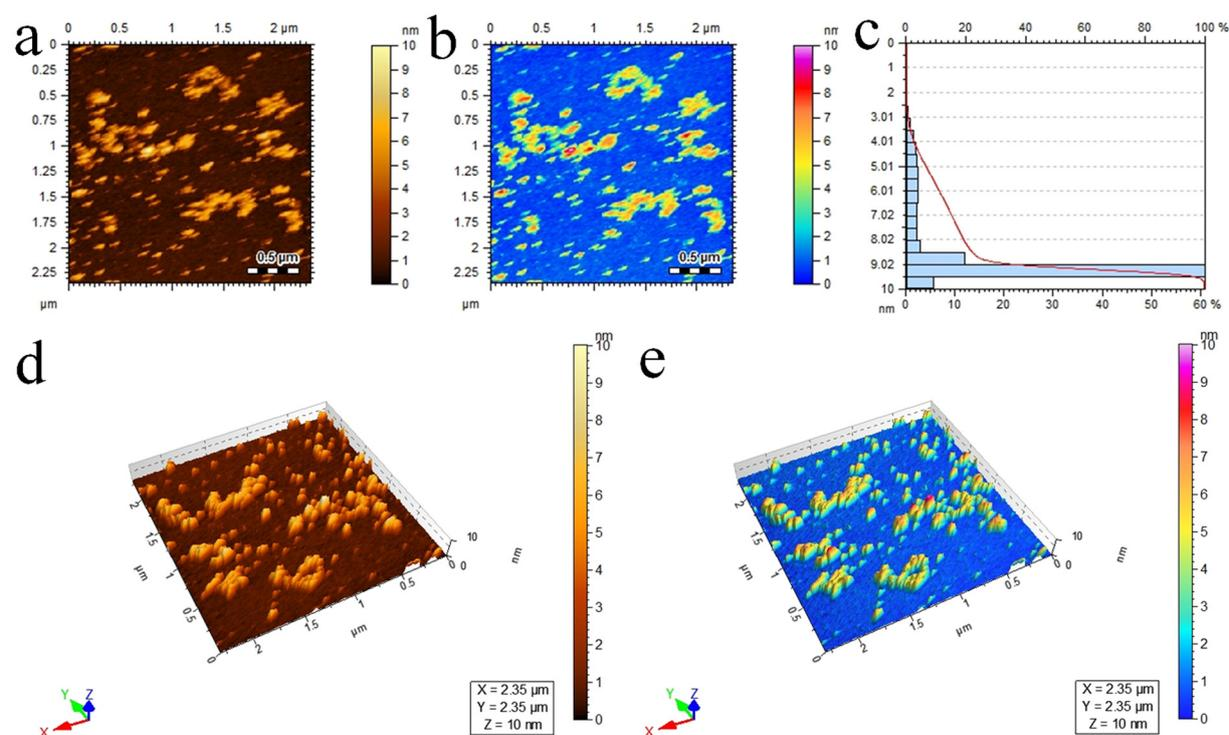
Fig. 5 AFM results of Pd@Ti<sub>3</sub>C<sub>2</sub>T<sub>x</sub>-TiO<sub>2</sub> photocatalysts: (a) and (b) 2D-tapping modes, (c) size distribution and (d) and (e) 3D images.
