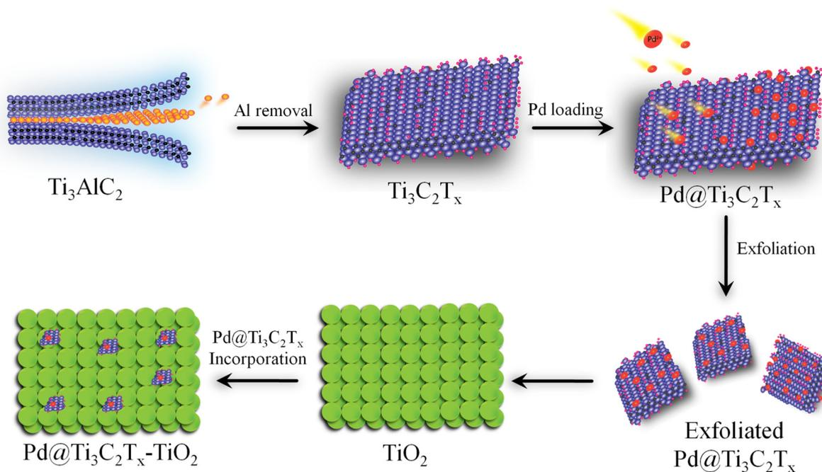
Fig. 1 Synthesis scheme of the Pd@Ti<sub>3</sub>C<sub>2</sub>T<sub>x</sub>-TiO<sub>2</sub> catalyst.
