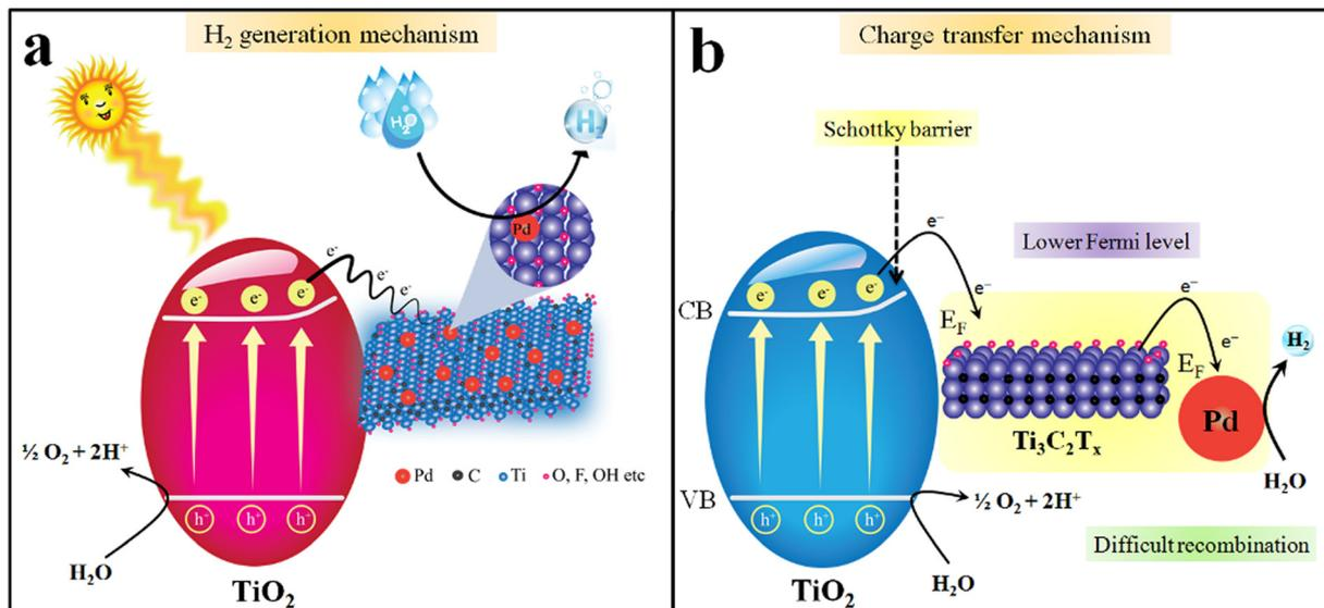
Fig. 10 Mechanism of (a) H<sub>2</sub> generation. (b) Charge transfer via Pd@Ti<sub>3</sub>C<sub>2</sub>T<sub>x</sub>-TiO<sub>2</sub>.
