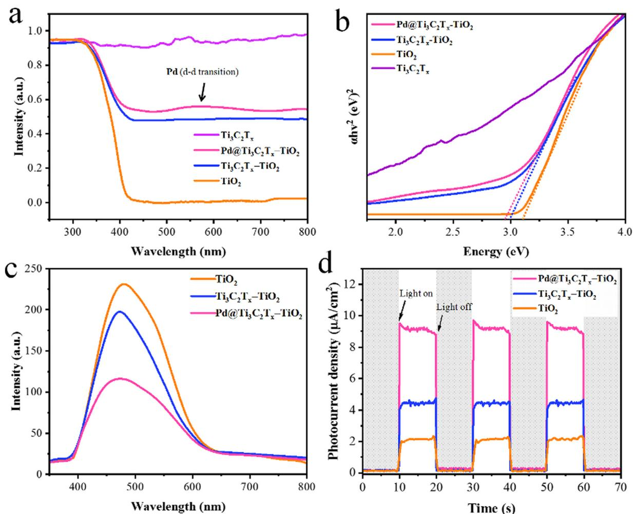
Fig. 7 (a) The UV-vis/DRS and (b) energy diagram of  $\text{TiO}_2$ ,  $\text{Ti}_3\text{C}_2\text{T}_x$ ,  $\text{Ti}_3\text{C}_2\text{T}_x\text{-TiO}_2$  and  $\text{Pd@Ti}_3\text{C}_2\text{T}_x\text{-TiO}_2$ . (c) and (d) PL and photocurrent density of  $\text{TiO}_2$ ,  $\text{Ti}_3\text{C}_2\text{T}_x\text{-TiO}_2$ , and  $\text{Pd@Ti}_3\text{C}_2\text{T}_x\text{-TiO}_2$ .
