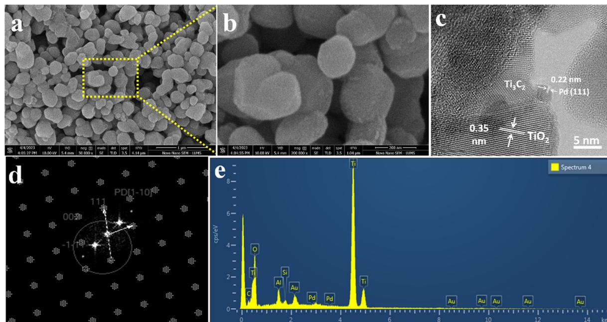
Fig. 4 SEM images at (a) 1  $\mu\text{m}$  and (b) 200 nm, (c) HR-TEM, (d) TEM diffraction pattern, and (e) EDX analysis of Pd@Ti<sub>3</sub>C<sub>2</sub>T<sub>x</sub>-TiO<sub>2</sub>.
