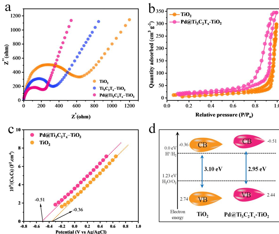
Fig. 8 (a) EIS results of TiO<sub>2</sub>, Ti<sub>3</sub>C<sub>2</sub>T<sub>x</sub>-TiO<sub>2</sub> and Pd@Ti<sub>3</sub>C<sub>2</sub>T<sub>x</sub>-TiO<sub>2</sub>. (b) BET results, (c) Mott-Schottky and (d) calculated band positions of TiO<sub>2</sub> and Pd@Ti<sub>3</sub>C<sub>2</sub>T<sub>x</sub>-TiO<sub>2</sub>.
