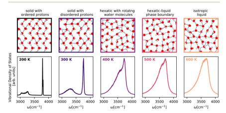
Fig. 5 Temperature-dependent vibrational density of states of monolayer water<sup>25</sup> across the solid-hexatic-liquid phase transition at a lateral pressure of 1 GPa calculated using the  $T_e$  PIGS method. The spectra are colour-coded according to temperature. The top panels (border colours indicating temperatures) correspond to snapshots of monolayer water structures. All simulations are performed with a BPNN trained at the revPBE0-D3 level of theory.
