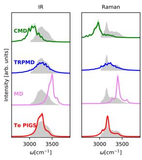
Fig. 3 IR and Raman stretching band of polycrystalline ice at 150 K with the  $T_{\rm e}$  PIGS (red), MD (pink), TRPMD (blue), and CMD (green) and the experimental spectra<sup>92</sup> (shifted by  $22~{\rm cm}^{-1}$  to account for the missing quantum coherence effects in simulation methods) in grey. All simulations are performed with a BPNN with SPC charges trained at the revPBE0-D3 level of theory.
