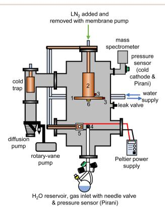
Fig. 1 Schematic illustration of the experimental setup used for the cryogenic codeposition of adamantane and water vapour. The components inside the chamber are (1) liquid-nitrogen cooled and removable 8-inch diameter copper plate, (2) liquid nitrogen reservoir, (3) K-type thermocouples, (4) metal mesh covering the water vapour inlet tube, (5) Peltier element with copper sample stage and pellet of either  $C_{10}H_{16}$  or  $C_{10}D_{16}$  and (6) quartz crystal microbalance.
