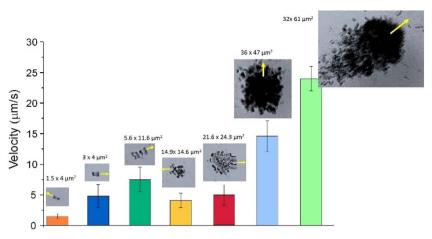
Fig. 6 Average velocity measured for individual Nafion-based swimmers and Nafion clusters of different sizes. The characteristic dimensions of the Nafion ensembles are indicated in the figure, together with the swimming direction of the collective structure.
