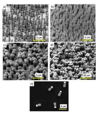
Fig. 5 Scanning electron microscope images of different Nafion arrays generated by colloidal lithography with the RIE technique. In (a) and (b) microparticles with diameters of  $1\,\mu m$  have been used as masks and 0.1 and 0.2% of particle dispersions, respectively. In (c) and (d)  $2\,\mu m$  diameter microparticles have been used as masks and 0.2% of particle dispersions but different RIE times (3 and 4 minutes, respectively). (e) Dispersed particles after an ultrasonic bath.
