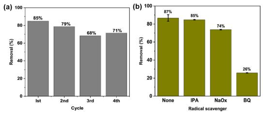
Fig. 6 (a) Percentage of TET removal upon C600KT recycling and (b) effect of radical scavengers on TET removal from aqueous solution with C600KT after 60 min. Fig. 6a does not have error bars because each bar represents a single experiment. The error bars in Fig. 6b are small showing a high reproducibility.
