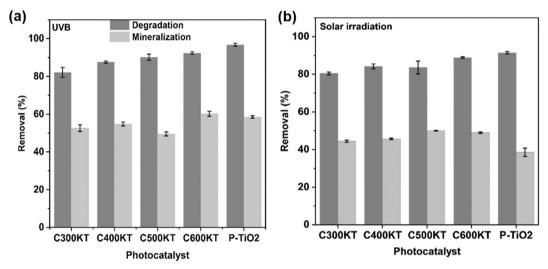
Fig. 7 Mineralization and degradation of TET in aqueous solution by P-TiO<sub>2</sub> and all composites under (a) UVB and (b) solar irradiation for 120 min. Dark grey is degradation, light grey indicates mineralization in both panels.
