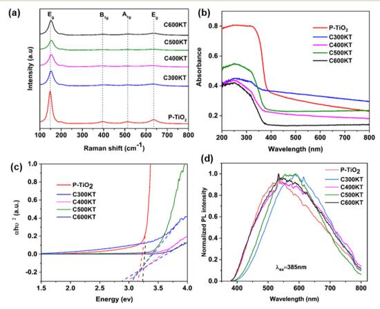
Fig. 2 (a) Raman spectra, (b) UV-vis DRS spectra, (c) Tauc plot analysis, and (d) PL spectra of  $P-TiO_2$  and all NCs. Raman spectra in panel (a) are shifted vertically for clarity. Band gaps calculated from Fig. 1c are shown in Table 1.
