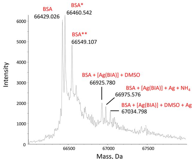
**Fig. 1** Deconvoluted mass spectrum of BSA,  $C_{\text{BSA}} = 1.00 \mu\text{M}$ , in the presence of  $2.00 \mu\text{M}$  of  $[\text{Ag}(\text{BIA})_2]^+$  in  $20 \text{ mM NH}_4\text{OAc}$  solution,  $\text{pH} = 6.8$ .  $0.1\% \text{ v/v}$  of formic acid was added just before injection into the mass spectrometer. BSA\* = sulfinylation on Cys34; BSA\*\* = cysteinylolation on Cys34.<sup>35</sup>
