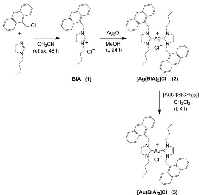
**Scheme 1** Synthesis of bis(1-(anthracen-9-ylmethyl)-3-butylimidazol-2-ylidene) silver chloride  $[\text{Ag}(\text{BIA})_2]\text{Cl}$  (2) and bis(1-(anthracen-9-ylmethyl)-3-butylimidazol-2-ylidene) gold chloride  $[\text{Au}(\text{BIA})_2]\text{Cl}$  (3).
