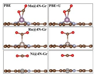
Fig. 3 CO<sub>2</sub> adsorption on TM@4N-Gr: chemisorption versus physisorption. Left: PBE; right: PBE+U.
