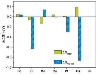
Fig. 6 Deviation of Gibbs free energies computed at PBE and PBE+U levels for H<sub>2</sub>O adsorption (green) and CO<sub>2</sub> co-adsorption (blue) in the presence of \*H<sub>2</sub>O on TM@4N-Gr.
