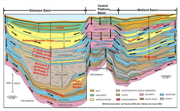
Fig. 12 A cross-section of the Delaware, Central Platform, and Midland sub-basins.<sup>79</sup>
