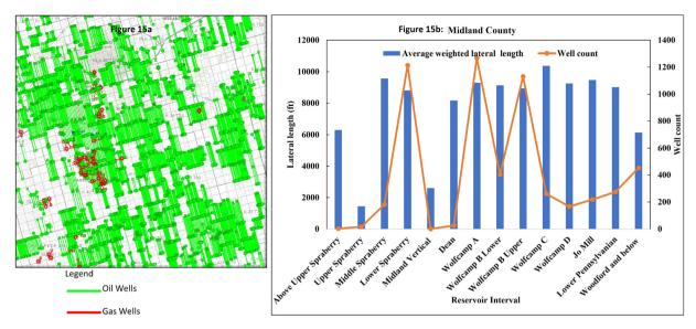
Fig. 15 (a) Map of Midland County area, Texas, showing the distribution of horizontal wells. (b) Reservoir interval with the lateral-length distribution per layer and well count.
