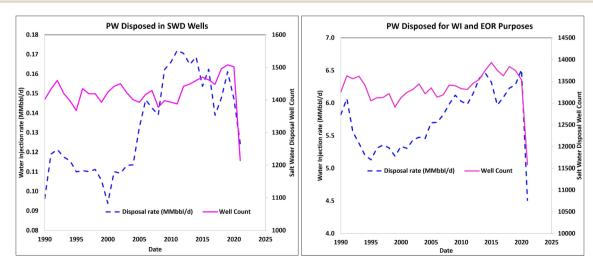
Fig. 19 Historic water-injection rates either for disposal or oil and gas recovery purposes.
