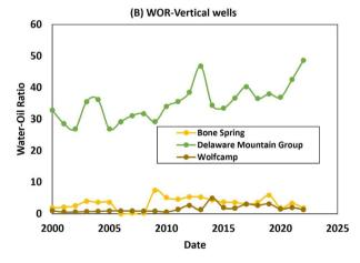
Fig. 7 Comparison of the WOR historical profile for (a) horizontal and (b) vertical well producing from similar reservoir systems for selected examples (data source Enverus drilling info).
