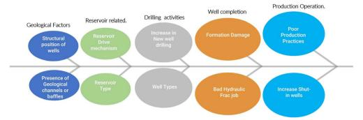
Fig. 4 Factors controlling the volume of water production.
