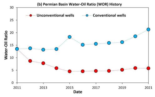
Fig. 9 (a) Disposed water volumes from conventional and unconventional wells by county as of December 2021. (b) Historic produced WOR of the Permian Basin.
