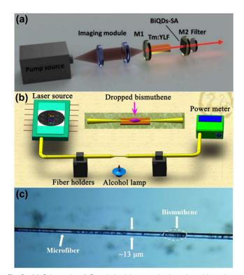
Fig. 9 (a) Schematic of Q-switched laser cavity based on bismuthene quantum dots. Reprinted with permission from Elsevier. 78 (b) Schematic diagram of the experimental setup for the fabrication of a microfiber. Reprinted with permission from ACS Publications. 96 (c) Microscopy image of the prepared microfiber saturable absorber based on bismuthene. Reprinted with permission from ACS Publications. 96
