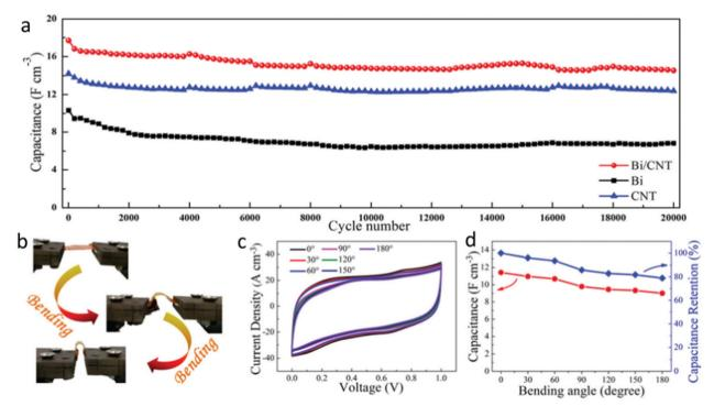
Fig. 10 (a) Cycling performance of capacitance for Bi/CNTs, Bi and CNTs at a scan rate of 0.5 V s<sup>-1</sup>. (b) Photographs of Bi/CNTs tested under different bending angles. (c) CV curves obtained at different bending angles, at  $0.5 \text{ V s}^{-1}$ . (d) Volumetric capacitance and capacitance retention as a function of bending angle. Reprinted with permission from RSC. 106
