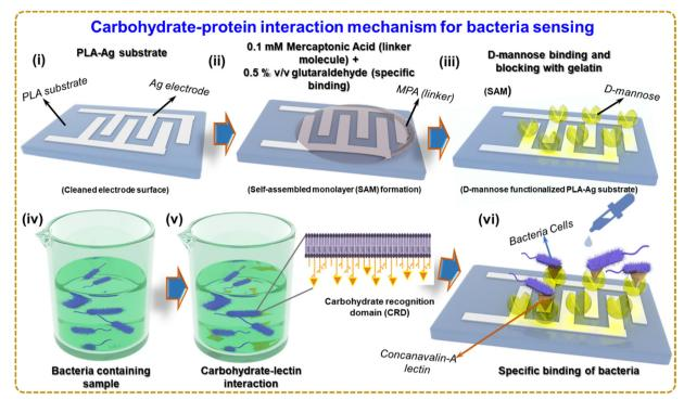
Fig. 4 Carbohydrate protein interaction mechanism of bacteria sensing (i) PLA-Ag substrate, (ii) self-assembled monolayer (SAM) formation, (iii) p-mannose functionalized substrate, (iv) and (v) bacteria containing sample and carbohydrate-lectin interaction. (vi) Specific binding of bacteria.
