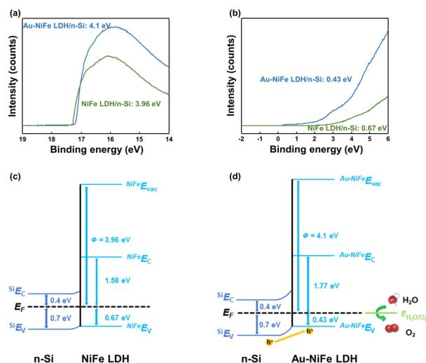
Fig. 5 (a) The secondary electron emission spectra of Au-NiFe LDH/n-Si and NiFe LDH/n-Si. (b) Valence band spectra ( $E_F - E_{VBM}$ ) of Au-NiFe LDH/n-Si and NiFe LDH/n-Si. Energy band diagram schematics of the (c) NiFe LDH/n-Si and (d) Au-NiFe LDH/n-Si.
