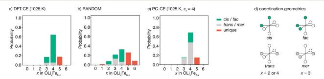
Fig. 2 (a–c) Oxygen coordination environment probability distributions for  $Li_2$ FeSO for (a) a density-functional theory derived cluster expansion model (DFT-CE), from Monte Carlo simulations at 1025 K, (b) random Li/Fe positions (RANDOM), and (c) an on-site point-charge cluster expansion model (PC-CE), from Monte Carlo simulations at 1025 K. (d) Schematic of *cis versus trans* (top) and *fac versus mer* (bottom) pseudo-octahedral coordination environments.
