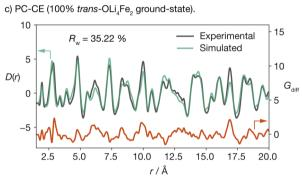
Fig. 3 Comparison of pair-distribution functions (PDFs) obtained from X-ray total scattering and simulated PDF data for Li<sub>2</sub>FeSO for structural models generated for (a) the DFT-fitted cluster-expansion model (DFT-CE), (b) the RANDOM model, and (c) the PC-CE point-charge model
