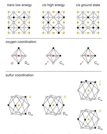
Fig. 5 Illustration of the three structures of interest (top) with their oxygen (middle) and sulfur (bottom) environments shown with them. For the illustrated coordination environments, polar coordination environments are marked with an arrow and non-polar environments are marked with a crossed square.
