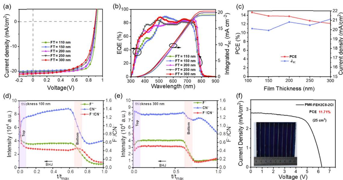
Fig. 5 (a)  $J$ - $V$  curves and (b) EQE curves of the conventional structure. (c) The PCE and  $J_{sc}$  of different film-thickness devices. (d and e) TOF-SIMS ion yield of  $F^-$  and  $CN^-$  of (d) 100 nm and (e) 300 nm film devices. (f) The image and  $J$ - $V$  curves of solar modules based on PM6:FEH2C8-2Cl film with an active layer of 25 cm<sup>2</sup>.
