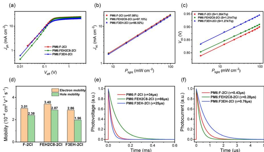
Fig. 3 (a) Plots of  $J_{ph}$  vs.  $V_{eff}$  for F-2Cl-, FEH2C8-2Cl-, and F3EH-2Cl-based OSCs. (b)  $J_{sc}$  characteristics of F-2Cl-, FEH2C8-2Cl-, and F3EH-2Cl-based OSCs under different light densities. (c)  $V_{oc}$  characteristics of F-2Cl-, FEH2C8-2Cl-, and F3EH-2Cl-based OSCs under different light densities. (d) Charge mobilities histogram. (e) TPV and (f) TPC of F-2Cl-, FEH2C8-2Cl-, and F3EH-2Cl-based OSCs.
