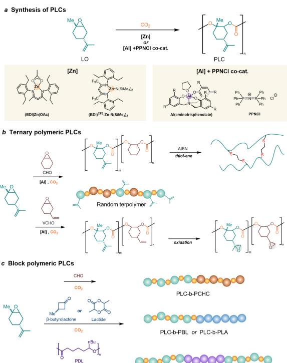
Fig. 5 The synthesis and copolymerization of PLCs. (a) The synthesis of PLCs *via* metal catalysts [Zn] or [Al]; (b) ternary polymeric PLCs synthesis by randomly adding LO and multiple epoxide monomers; (c) the synthesis of block polymer PLCs.
