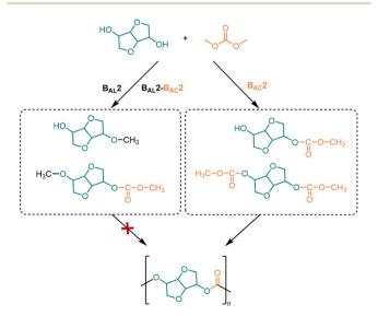
Fig. 3 DMC-induced mechanism to synthesize PICs.
