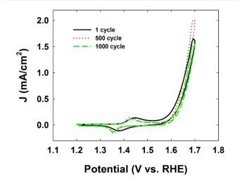
Fig. 2 Cyclic voltammograms of Ni-CN-200 modified electrode for the durability test after 500 or 1000 cycles at a scan rate of  $100 \, \mathrm{mV} \, \mathrm{s}^{-1}$ . The electrolyte solution was Ar-saturated 1 M KOH [reproduced from ref. 25, with kind permission].
