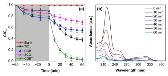
Fig. 5 (a) Photocatalytic degradation of PCP under photolysis and in the presence of catalysts:  $TiO_2$ , SCG, CGB, and CGBT nanocomposite, and (b) temporal band changes in absorbance spectra of PCP during photocatalytic degradation by CGBT nanocomposites. [(PCP)<sub>o</sub> = 10 mg L<sup>-1</sup>, catalyst dosage of 1 g L<sup>-1</sup>, pH 5, and UV light irradiation).
