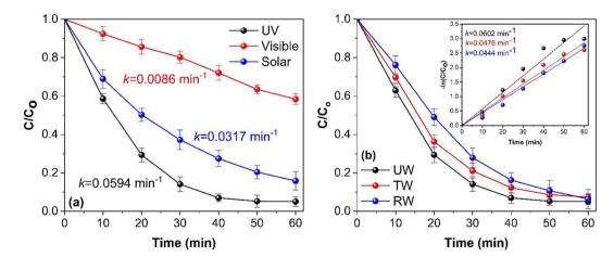
Fig. 6 (a) Effect of different light sources and (b) water matrix on the photocatalytic degradation of PCP (inset: rate kinetics).  $[(PCP)_0 = 10 \text{ mg L}^{-1}, PCP]_0 = 10 \text{ mg L}^{-1}$ CGBT dosage of 1 g  $L^{-1}$ , pH 5, and UV light irradiation).
