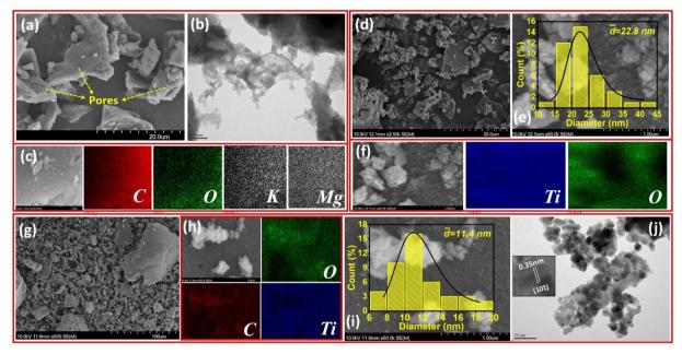
Fig. 1 (a) SEM image, (b) TEM image, and (c) EDS maps of spent-coffee ground biochar (CGB); (d) SEM image, (e) particle size distribution and (f) EDS maps of TiO<sub>2</sub>; and (q) SEM image, (h) EDS mapping, (i) particle size distribution and (j) TEM image of CGBT nanocomposites.
