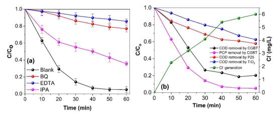
Fig. 7 (a) Effect of radical trapping experiments on the photocatalytic degradation of PCP, and (b) the removal of COD and the generation of  $Cl^-$  obtained during the photocatalytic degradation of PCP. [(PCP)<sub>o</sub> = 10 mg  $L^{-1}$ , CGBT and  $TiO_2$  dosage of 1 g  $L^{-1}$ , pH 5, and UV light irradiation).
