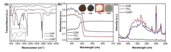
Fig. 3 (a) FT-IR spectra, (b) UV-vis DRS analysis (inset: picture of powder form of spent-coffee grounds (SCG), coffee-grounds biochar (CGB), TiO<sub>2</sub>, and coffee-ground biochar-supported TiO<sub>2</sub> nanocomposites (CGBT)), and (c) photoluminescence spectra of the synthesized materials.
