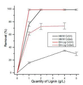
Fig. 9 Reduction and removal of Cr(vi) and Cr(tot) using different quantities of EH and HMW under reference conditions.
