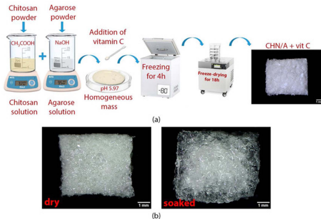
Fig. 9 (a) The preparation of the CHN/A + vit C biomaterial. (b) Dry and hydrated material. (b) The exceptional ability of the material to remain intact in the presence of water makes it beneficial in wound treatment. 109
