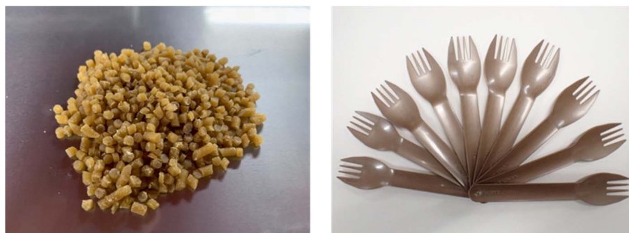
Fig. 42 100% biomass biodegradable resin pellet (Left) and forks (Right) made from Sargassum waste.
