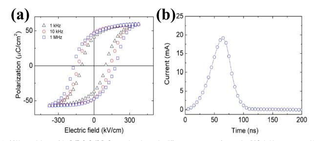
Fig. 3 (a) Hysteresis loops of the Pt/ZnSnO<sub>3</sub>/SrRuO<sub>3</sub> capacitor observed at different measurement frequencies. (b) Switching-current as a bias of 5 V. The fast-switching behaviour is within 100 ns.<sup>49</sup>
