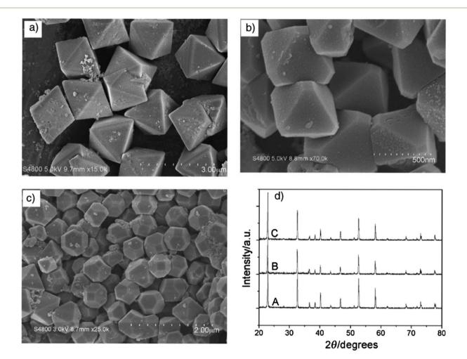
Fig. 12 Typical SEM images of the as-prepared ZnSnO<sub>3</sub> products: (a) CTAB 0.15 M, (b) CTAB 0.4 M, and (c) CTAB 0.75 M. (d) Corresponding XRD patterns of the as-prepared ZnSnO<sub>3</sub> polyhedra, (A) octahedra, (B) truncated octahedra and (C) 14-faceted polyhedra.<sup>102</sup>
