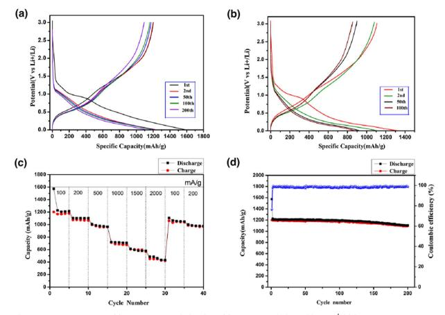
Fig. 20 Charge–discharge profiles of (a) sandwich-like ZnSnO<sub>3</sub>@C and (b) sheet-like ZnSnO<sub>3</sub> at 100 mA  $g^{-1}$ . (c) Cycling activity at various current densities. (d) Cycling activity at 100 mA  $g^{-1}$  of the sandwich-like ZnSnO<sub>3</sub>@C.<sup>194</sup>
