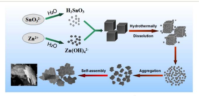
Fig. 10 Diagram depicting the probable process for the formation of the precursor ZnSn(OH)<sub>6</sub>.<sup>95</sup>
