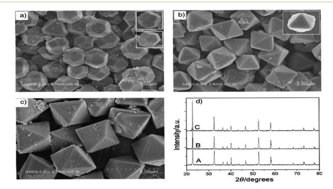
Fig. 11 SEM micrograph of ZnSnO<sub>3</sub> obtained using: (a) SDBS 0.15 M, (b) SDBS 0.4 M, and (c) SDBS 0.75 M. (d) XRD pattern of (A) 14-faceted polyhedra, (B) truncated octahedra and (C) octahedra.<sup>102</sup>
