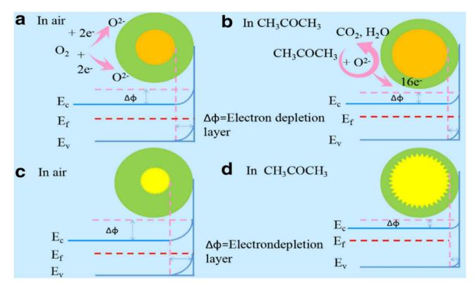
Fig. 18 Schematic band diagrams of ZnSnO<sub>3</sub> hollow microspheres exposed to (a) air and (b) CH<sub>3</sub>COCH<sub>3</sub>, and ZnSnO<sub>3</sub>/SnO<sub>2</sub> hollow urchin gas sensors exposed to (c) air and (d) CH<sub>3</sub>COCH<sub>3</sub>.<sup>218</sup>
