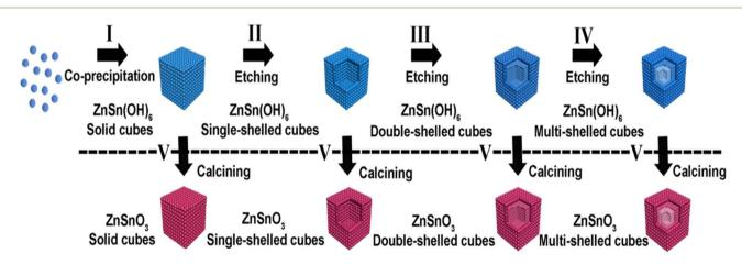
Fig. 15 Schematic illustration of the fabrication of ZnSnO<sub>3</sub> hollow-boxes under basic-etching and calcination.<sup>129</sup>
