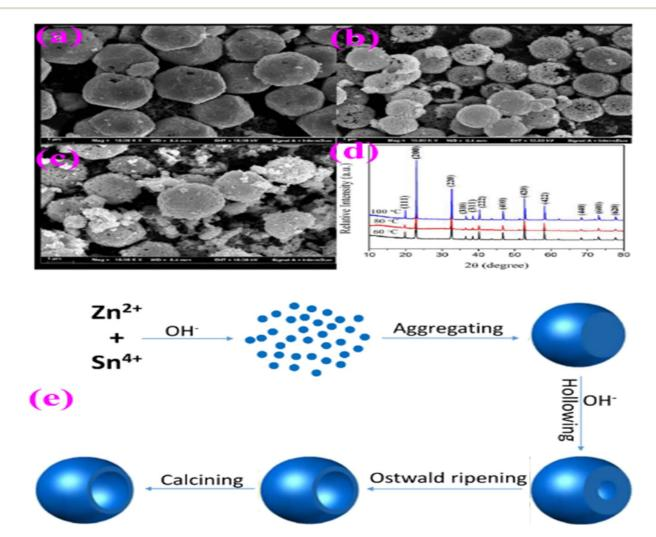
Fig. 14 SEM images of  $ZnSnO_3$  obtained at different reaction temperatures: (a) 60 °C, (b) 80 °C, and (c) 100 °C. (d) XRD patterns of  $ZnSn(OH)_6$  precursor. (e) Schematic illustration of the possible formation mechanism of  $ZnSnO_3$  hollow spheres.<sup>70</sup>
