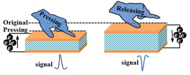
Fig. 23 Working mechanism of generating power from a piezoelectric nanogenerator.<sup>215</sup>
