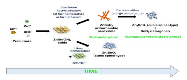
Fig. 1 Schematic illustration of phase rearrangements during the hydrothermal process of zinc stannate nanostructures as a function of reaction energy and synthesis time.<sup>34</sup>
