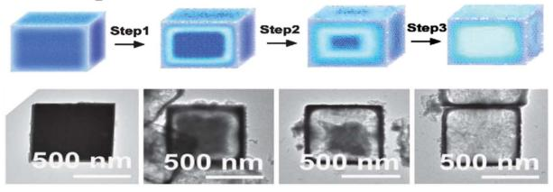
Fig. 16 Potential mechanism illustrating the acid etching process and the resulting synthesized products when employing cubic  $ZnSnO_3$ templates.92
