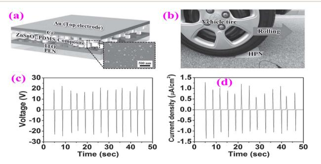
**Fig. 22** Structure and power generation by HP-NG when a tire is rolled. (a) Illustration of the structure of the ZnSnO<sub>3</sub>:PDMS nanocompositebased flexible HP-NG as seen by the cross-sectional FESEM image. (b) Experimental setup for power production under the rolling of a vehicle tire, in which ZnSnO<sub>3</sub>:PDMS HP-NG was attached to the road. (c) Output voltage and (d) current density from HP-NG induced by the loading and unloading of a vehicle tire.<sup>214</sup>
