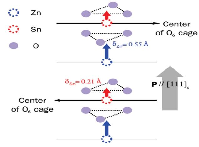
Fig. 4 Ionic rearrangements of Zn and Sn in the R3c phase of ZnSnO<sub>3</sub>.<sup>49</sup>
