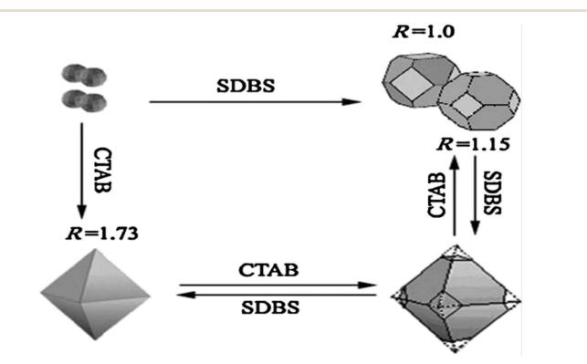
Fig. 13 Schematic diagram depicting the relationship between the ratio R and the transformation of the crystal shape.<sup>102</sup>
