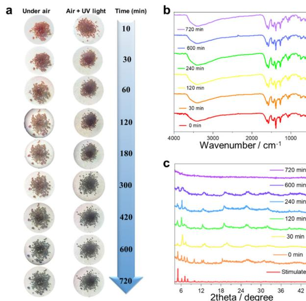
**Fig. 4** Color-change map of cluster 1 at different time points under the conditions of air and UV light exposure (a). FTIR spectra and PXRD patterns of cluster 1 at different time points in air (b and c).
