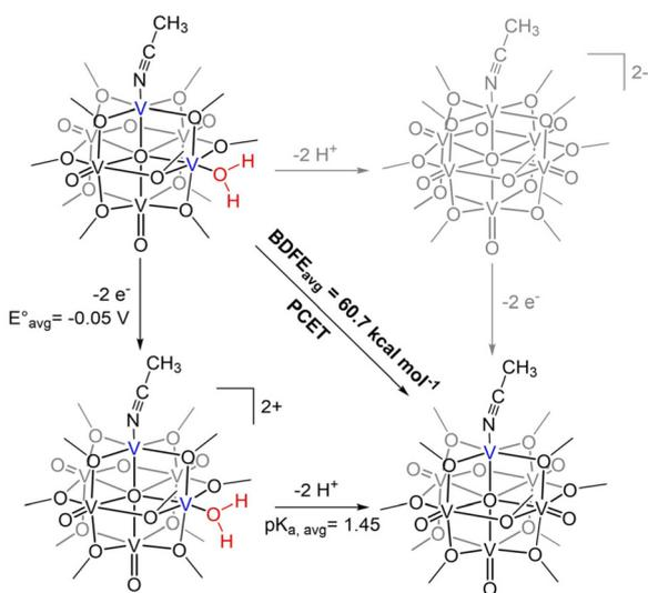
**Scheme 3** Square scheme of 2e<sup>-</sup>/2H<sup>+</sup> reduction of [V<sub>6</sub>O<sub>6</sub>(OH<sub>2</sub>)]<sup>0</sup> to [V<sub>6</sub>O<sub>5</sub>(MeCN)(OH<sub>2</sub>)]<sup>0</sup>.
