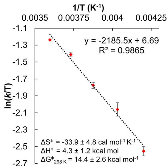
**Fig. 5** Eyring plot for the reaction of [V<sub>6</sub>O<sub>6</sub>(MeCN)]<sup>0</sup> (0.75 mM) with H<sub>2</sub>Phen (7.3 mM) in MeCN between -35 and 15 °C. Y-Axis values were determined by dividing *k*<sub>obs</sub> by the concentration of H<sub>2</sub>Phen, providing the rate constant, *k*<sub>PCET</sub>. Activation parameters are labelled on the plot.
