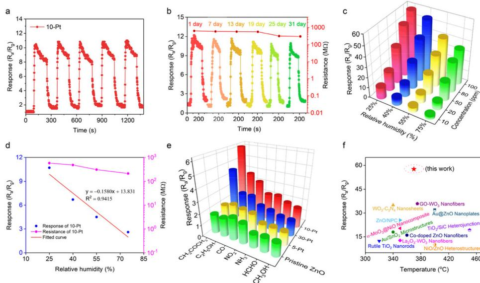
**Fig. 6** (a) Repeatability test and (b) long-term stability test of the 10-Pt sensor for 10 ppm acetone at 370 °C. (c) The response of the 10-Pt sensor to 10–100 ppm acetone at various relative humidity levels. (d) The variation of  $R_a$  and response values of the 10-Pt sensor versus relative humidity. (e) Selectivity test of the 10-Pt sensor to 5 ppm acetone at 370 °C. (f) Comparison of the gas-sensing performance of the 10-Pt sensor with that of the other SMO-based acetone sensors.
