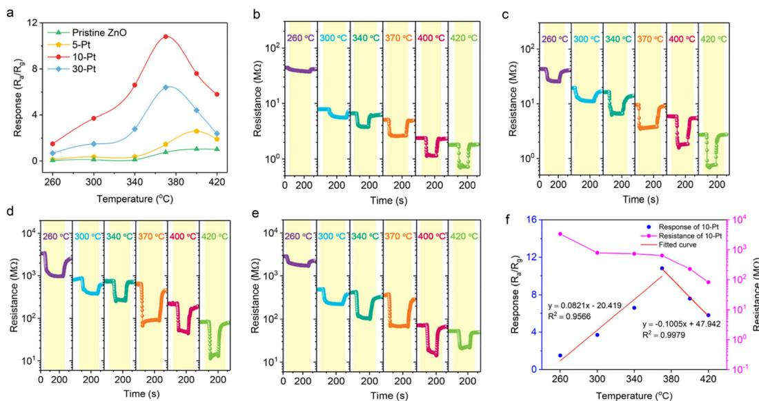
Fig. 4 (a) Response of the as-prepared samples to 10 ppm acetone at different temperatures. The transient change in  $R_a$  with operating temperature of (b) pristine ZnO, (c) 5-Pt, (d) 10-Pt and (e) 30-Pt sensors. (f) Response and  $R_a$  of the 10-Pt sensor to 10 ppm acetone around the working temperature.
