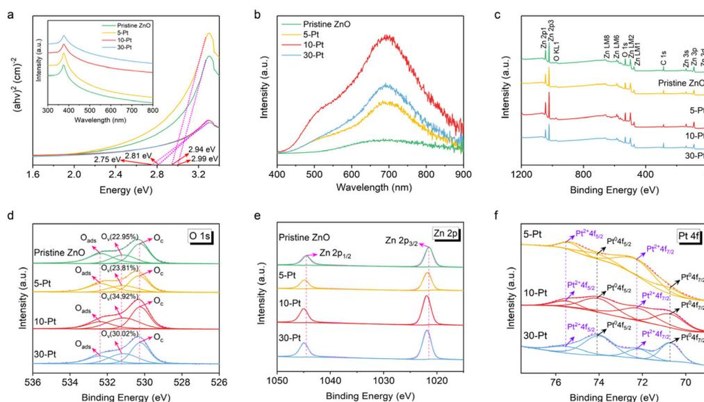
**Fig. 3** (a) Tauc plot and UV absorption spectra, (b) PL spectra, (c) survey XPS spectra, (d) O 1s XPS spectra and (e) Zn 2p XPS spectra of pristine ZnO, 5-Pt, 10-Pt and 30-Pt. (f) Pt 4f XPS spectra of 5-Pt, 10-Pt and 30-Pt.
