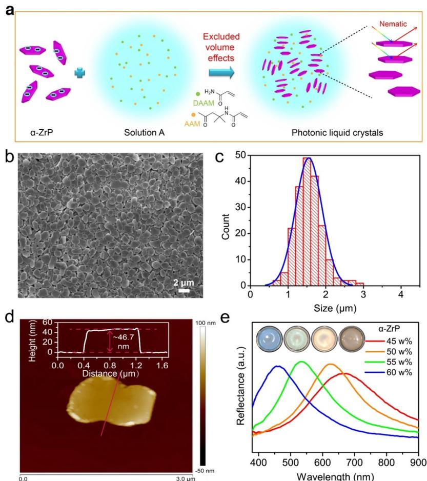
**Fig. 2** (a) SEM image and (b) lateral size distribution of the fractionated  $\alpha$ -ZrP nanoplates. (c) Schematic illustration showing preparation process of the photonic LC suspensions. (d) AFM image of  $\alpha$ -ZrP nanoplates, the inset is height profile. (e) Reflection spectra of the suspensions prepared with different mass fractions of  $\alpha$ -ZrP, the insets show the corresponding structural color variation.
